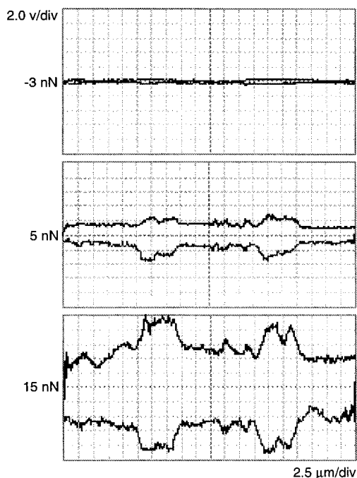
FIGURE 6 Friction “loops” demonstrating the friction hysteresis with increasing applied load. Here the modified tip is scanned back and forth in a line across a substrate containing regions of complementary ( thin stripes ) and noncomplementary ( thick stripes ) oligonucleotides. The friction force is half the observed hysteresis.
